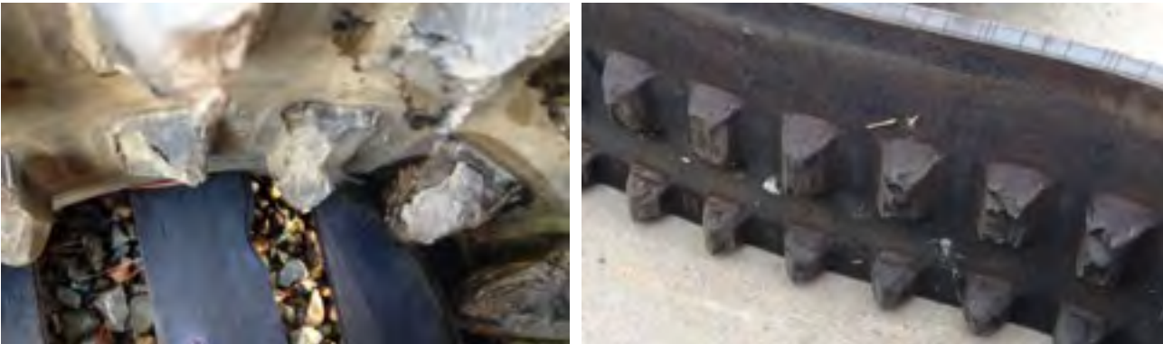
Drive Lug Loss Or Damage (jagged appearance or separation)
