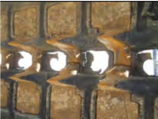
Big wear of the central due to operation on sandy field
