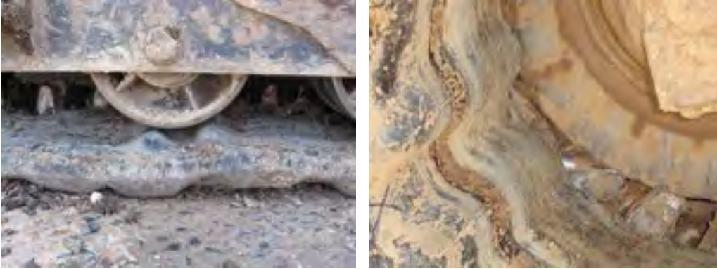
Early stage (Metal bars beginning to move in carcass)
