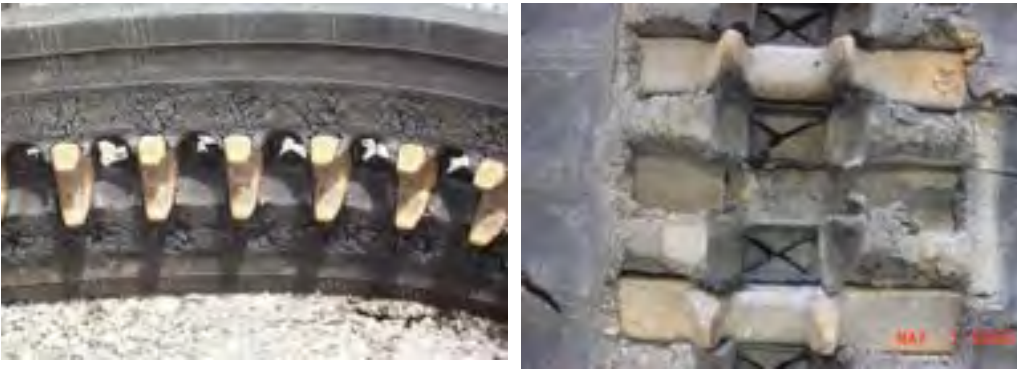
ID carcass wear (severe or rocky conditions)
