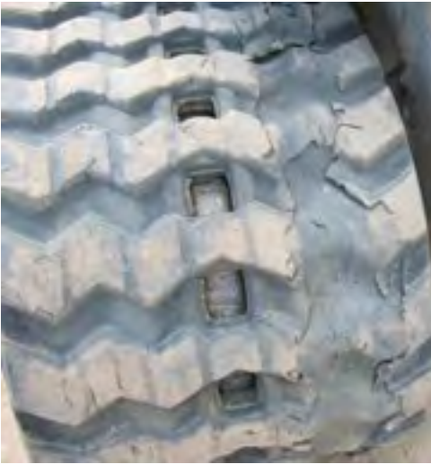
Delamination of layer
