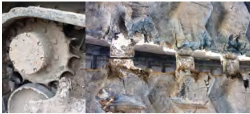
Breakage due to abraded sprocket
