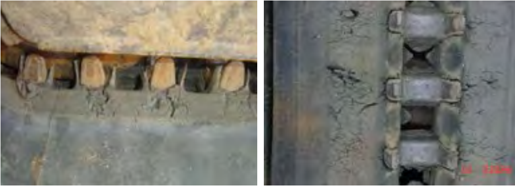
ID carcass wear (normal ground conditions)
