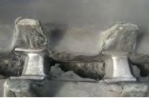
Big wear of the central due to non-adapted sprocket
